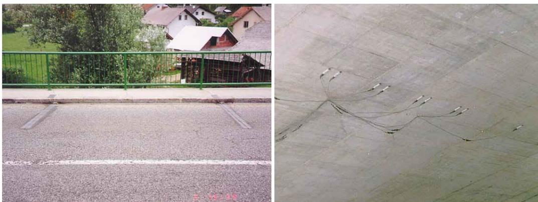
Figure 2: Pneumatic axle detectors on a bridge and strain transducers screwed on a bridge deck
