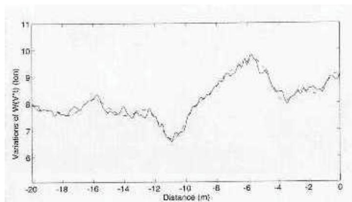
Figure 5: Variations of the impact force for the second axle of a 5-axle truck for  $n = 4$ , (—) experimental measurement, (---) reconstruction algorithm.
