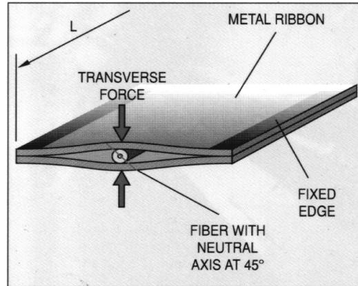
Figure 23: Sensitive element of the sensor
