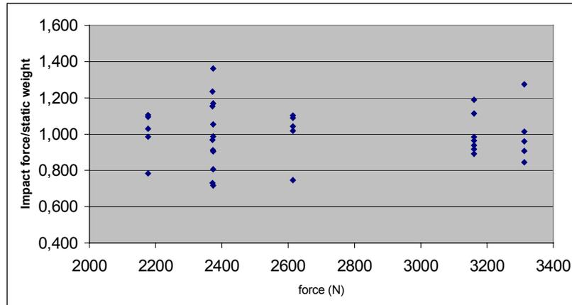
Figure 25: Comparison between impact force and static weight for a given force
