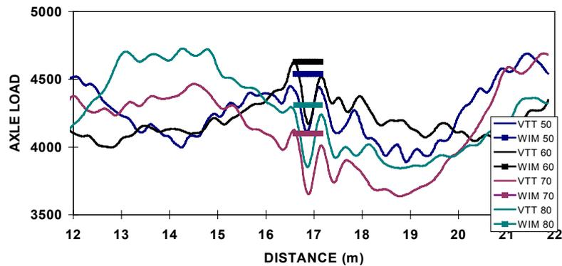
Figure 13: Dynamic axle loads of steering axle at four speeds; 50, 60, 70 and 80 km/h, and corresponding WIM-measurements
