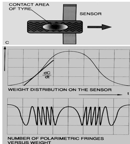
Figure 22: Example of typical signal from optical fibre sensor
