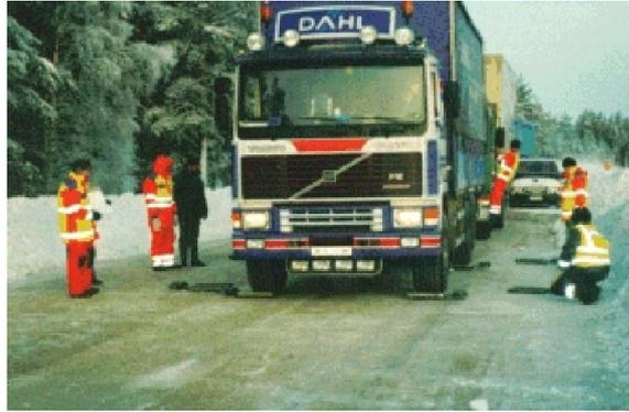
Figure 15: Static Weighing on Aleån test site in Sweden.
