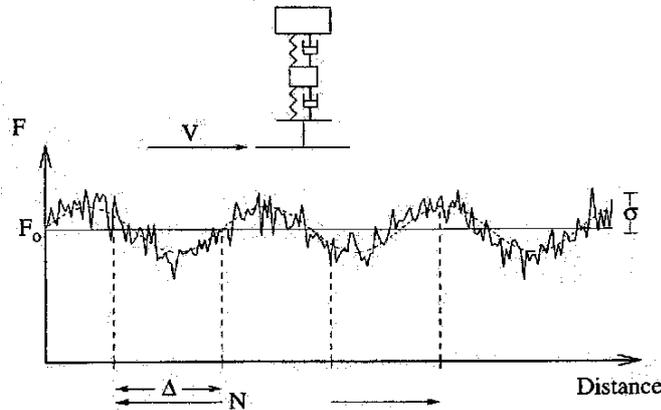
Figure 6: Impact force signal and design spacing
