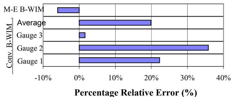
Figure 19: Comparison of results from multiple-equation (M-E) B-WIM and conventional B-WIM algorithms.
