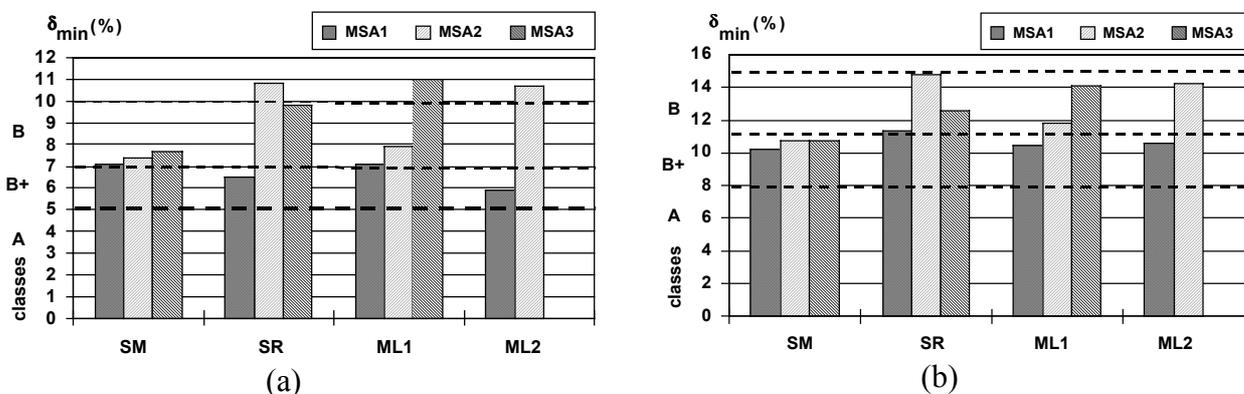
Figure 10: Estimation of Gross Weights (a) and Single Axles Loads (b) for a 2-axle rigid lorry (T2) and an articulated semi-trailer (T2R2) – Effects of sub-arrays
